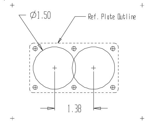
Note: The two 1.5 inch holes need to intersect to provide a channel for the dimmer/switch wiring. Drill the holes 1.38 apart on center.
