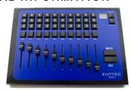
The Enttec Playback Wing is designed to allow fast, manual control of submasters in LightFactory and other PC-Based lighting control systems. It includes flash, next, pause, back, and go buttons, and has 99 pages of submasters available. The Enttec Playback Wing connects via Ethernet to your PC, meaning multiple Wings can be used if desired, and positioning is entirely up to the user. The Ethernet interface is plug and play, making it quick and simple to connect and get working!
