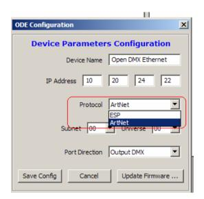
11. Assign your ODE to a Subnet and Universe in the Art-Net range of possible locations. If you only have one ODE, the default of 0,0 may be suitable, but when multiple devices are used then take care as to which you assign where, and consider labeling the outside of the box, perhaps with tape and a permanent marker, or by using a plastic stick-on label, so that you can deploy and troubleshoot it easily.
