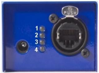
1 Status: This LED will blink when the ODE is operating normally. If the LED is on and does not blink it means the ODE is in fault, this could be due to a failed firmware upgrade. You may need to scan your network with NMU and re flash the firmware.
