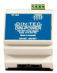
DIN-POWER offers 2 different power inputs, center positive 2.1mm DC Jack or Screw Terminal. You can use either one of these depending on the type of power supply you use.
