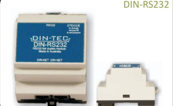
The DIN-RS232 is an RS232 to DIN-NET interface device. It can send RS232 strings when a particular DIN-NET action is received or send preprogrammed din-net actions when it receives an RS232 string matching a pre-programmed user defined string.
